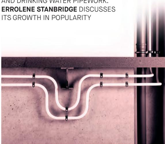
While copper and stainless steel are the traditional go-to materials for many building service systems, the properties of multilayer pipe can provide additional benefits such as a reduced number of fittings, minimal pressure loss and the ability to work in narrow areas.
