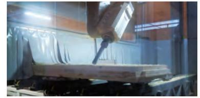
Precision-engineered timber components for schools could be manufactured using robotically aided CNC tools
